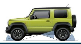
The ample approach angle of 37 degrees, ramp breakover angle of 28 degrees and departure angle of 49 degrees enables the Jimny to climb over obstacles and steep hills without the risk of scraping its bumpers or underbody.
