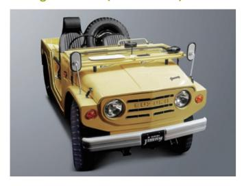
Development of the LJ10, Suzuki's first four-wheel drive lightweight vehicle, started in 1968. Developed to endure the rough usage of an off-roading vehicle, it went through a variety of severe tests, from dropping the vehicle one metre to the ground to testing durability in the volcanic sands of Mt. Fuji. It became available in the market in March 1970 and was the first mass-produced four-wheel drive in Japan's domestic mini-car category.
