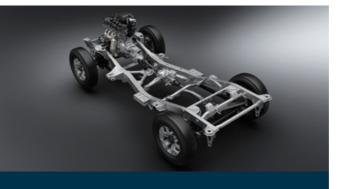
The ladder frame structure provides a solid base for suspension components when driving off-road and also helps protect the vehicle body even on bumpy surfaces. For the new Jimny, a new "x-member" and two additional cross members have been added for further reinforcement and increased torsional rigidity.
