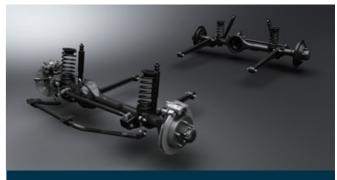
Rigid axle suspensions thrive in bumpy off-road driving. When one wheel is pushed upward by an obstacle, the connected wheel on the other side is pressed downward, giving superior grip on uneven terrain. The Jimny equips the rigid axle suspension layout on both the front and rear, allowing it to travel evenly on rough roads.
